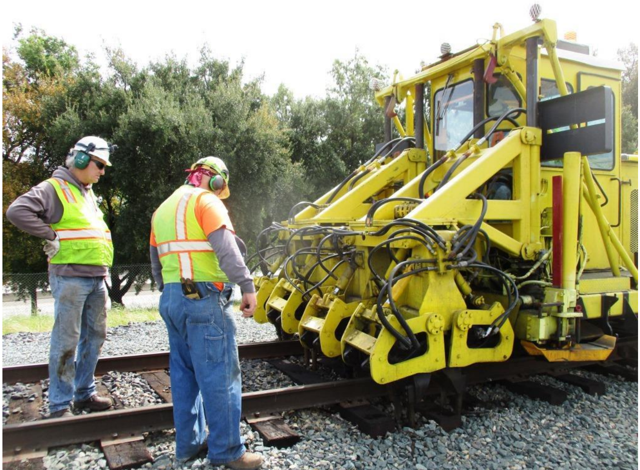
Steve and Mike F. work with Alan in the tamper to tamp low joints
