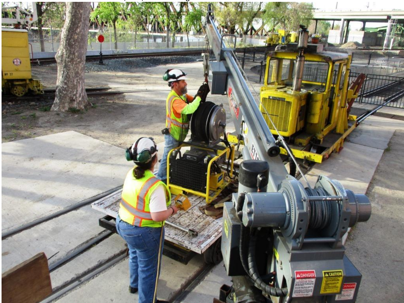
Heather and Joe use the MOW Truck's crane to lift the hydraulic power unit off the flatcar for its return to the Shops
